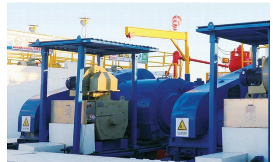
MOTOR-DRIVEN MUD PUMPS
